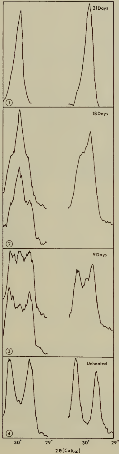
FIG. 5. Diffractometer traces of feldspars from pseudoleucite rocks (left) and traces of heat-treated Madagascar microcline (right). For explanation of groups 1 to 4 see text.
